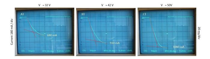
At the start of switch-on, a red gradient line can be drawn to indicate the value of di/dt occurring due to the inductance L  $\sim$  32V x 30ms /(3.5 x 180mA) = 1.52 H for plot A1, and similarly 42V x 30ms /(5.2 x 180mA) = 1.35 H for plot B1, and 50V x 30ms/(5.5 x 180mA) = 1.52 H for plot C1. Accuracy of inductance measurement is limited by the application of a gradient line estimate to the available plot data.
